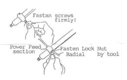
(3) Then, mount 2 Mount Brackets onto the Mount Support Pipe. Pass the coax. cable through the Pipe and connect to the Power Feeding Section. Please fasten Hex. Bolts firmly. Then, assemble such Support pipe to whole antenna and fasten Lock Bolt strongly.
